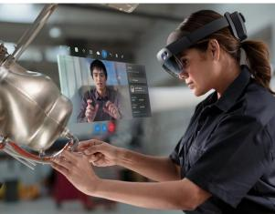
This technology allows the user to visualize 3D images projected in their immediate environment. Thanks to its array of sensors (movement, laser, etc.), the HoloLens 2 allows the user not only to see objects in 3D but also to manipulate them. The smart headset can be controlled both by voice commands and gestures, this being particularly relevant when working on our production lines.
