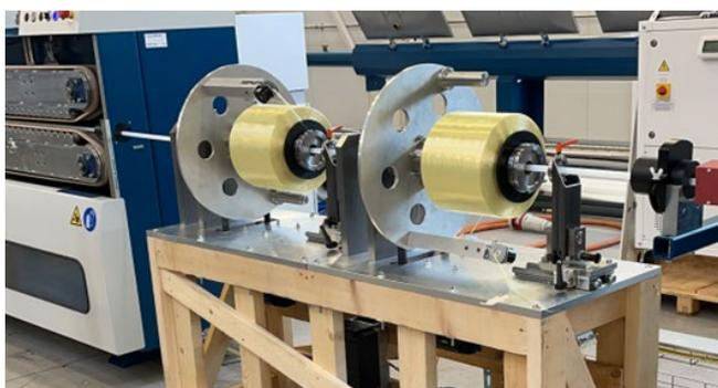
Double central binder test device in a MFWL063 line
