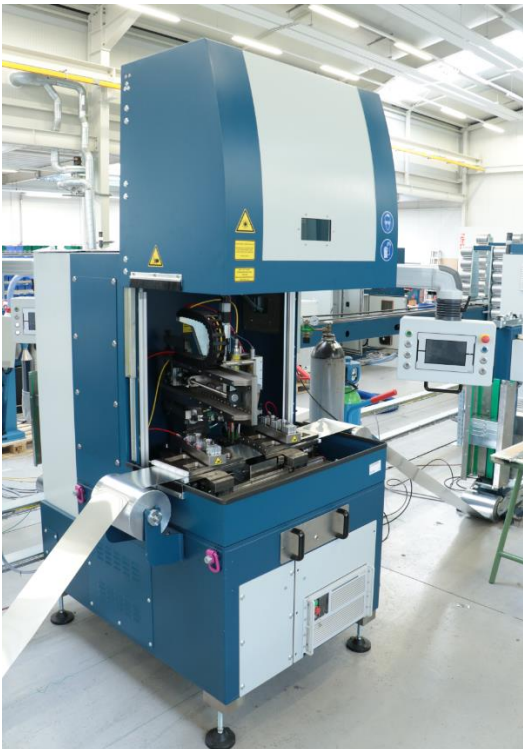
SLT 200 with 500 Watts, air cooled laser source
