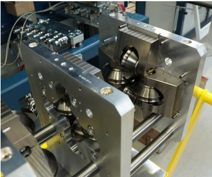
Fig. 3: Welding head and station VF
