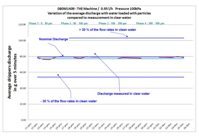
The classification of this emitter is **Non sensitive** to clogging. Consequently a **130 to 150 microns** filtration could suffice following the classification proposed by Irstea (according to the tests results with strictly mineral particles).
